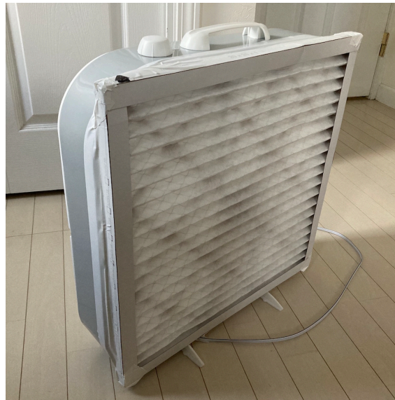
Fig.3 Completed photo of the air purifier we prototyped
